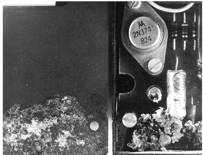
Figure 3-1. Corrosion Caused by Blown Capacitor Acid
